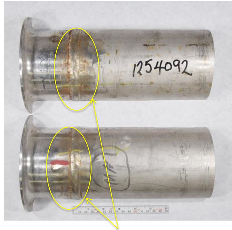
Significant Iron Contamination
