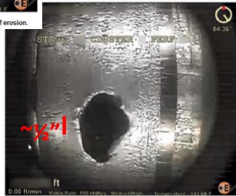
Figure 12—Post-Fracturing perforation image clearly showing significant erosion.
