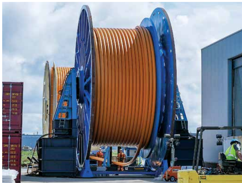
FIG. 1. TCP flowlines, similar to those shown here, will be headed to Africa for a supermajor. Image: Airborne Oil & Gas.
