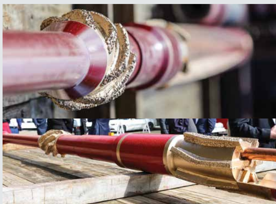
FIG. 1. The AlphaST single-trip, open-hole, cementing sidetrack system (top and bottom) saved one operator 29 hours of rig time and more than $100,000 of operational expense.
