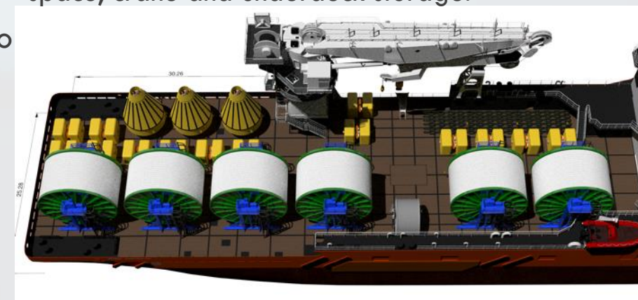
25m beam AHTS and OCV which has larger deck space, crane and underdeck storage.
