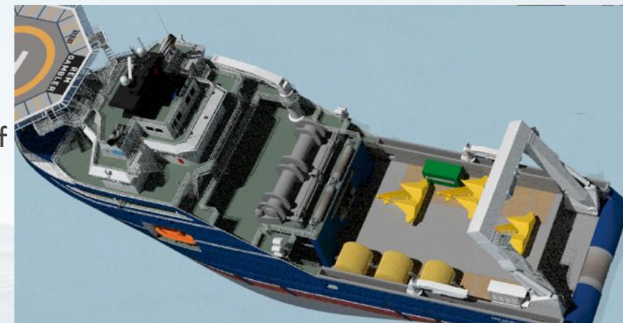
25m beam AHTS and OCV which has larger deck space, crane and underdeck storage.
